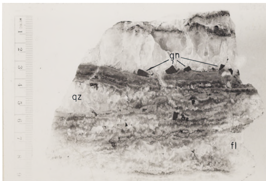
Figure 8. Typical "Coon Tail" ore from Mex-Tex mine. Contains galena cubes, banded silicified limestone, and crustiform quartz and fluorite. Galena (gn), Quartz (qz), Fluorite (fl).
